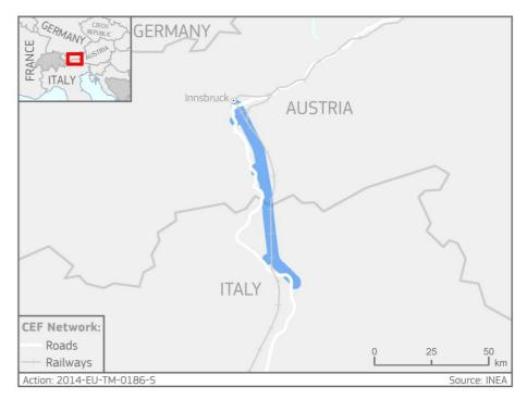
The Action is part of the Brenner Base Tunnel Global Project, centrepiece of the railway upgrade from Munich to Verona. As a low-gradient railway it will enable heavier and longer trains to operate on the line.
