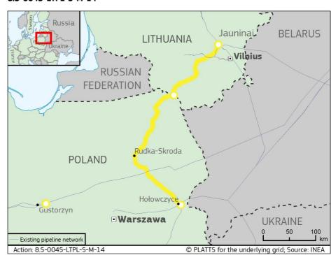
The Action contributed to the implementation of the Project of Common Interest (PCI) 8.5 Poland-Lithuania interconnection ("GIPL" or Gas Interconnection Poland-Lithuania), which is a gas pipeline that will connect the Polish and Lithuanian gas transmission systems.
