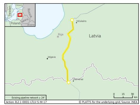
The Action contributed to the implementation of the Project of Common Interest (PCI) 8.2.1 Enhancement of Latvia-Lithuania, which aims to increase the interconnection capacity between the gas systems of both Member States.
