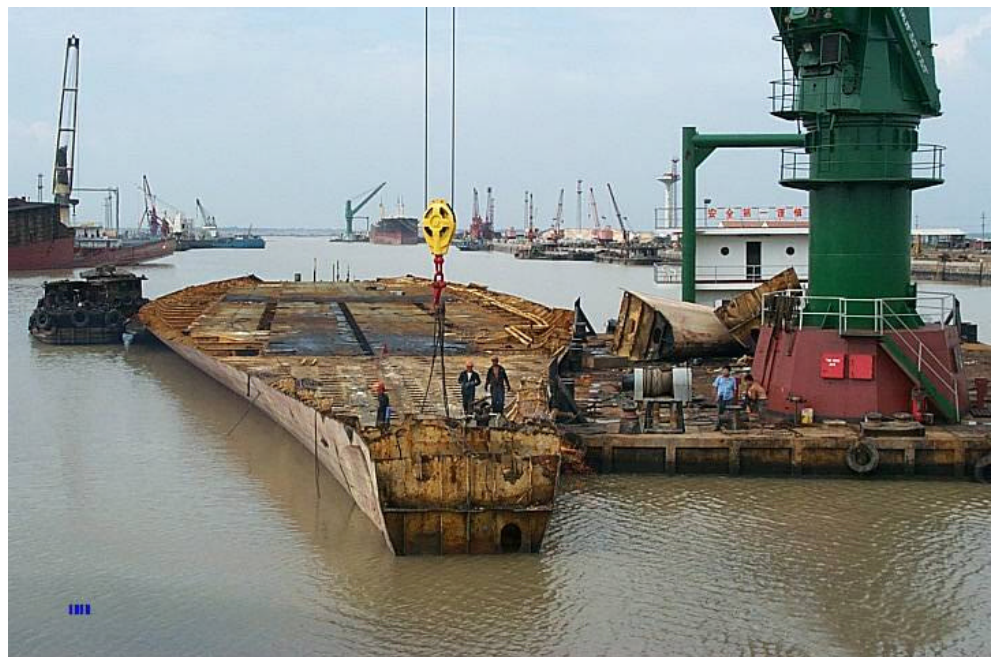
Keel to be broken up at Chinese yard (courtesy of T. Blankestijn, P&O Nedlloyd)
