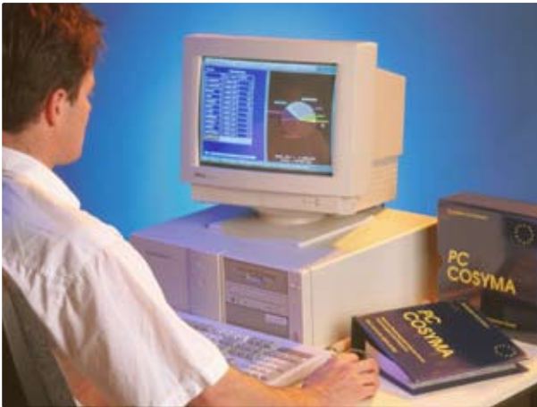
A desktop personal computer has a visual display unit incorporating a cathode ray tube.
