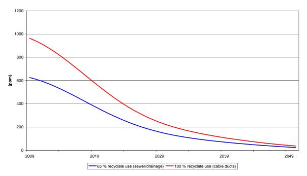
Cadmium concentration in new pipes
