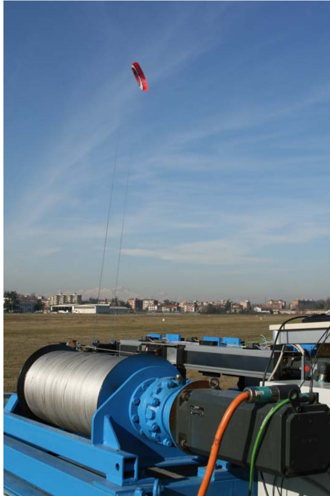
Figure 4: KG-yoyo small scale prototype operating near Torino, Italy.
