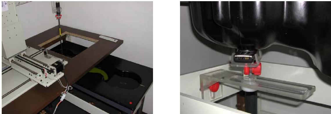
Fig. 2.16 SAR measurement system with liquid phantom and 3-D motor driver system.
