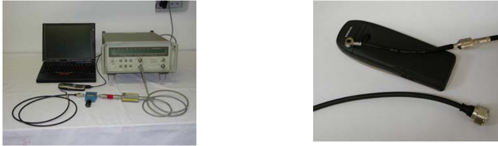
Fig. 2.13. Power measurements (left) and the external RF output and cable on the phone (right)
