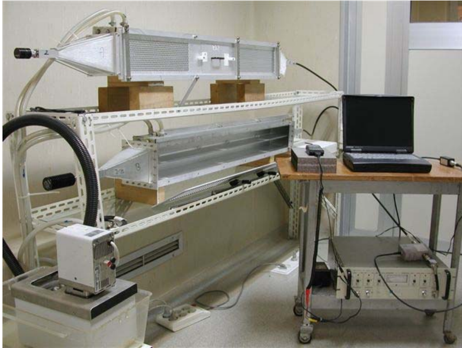
Fig. 2.8b TEM cell for actual exposure and sham experiments
