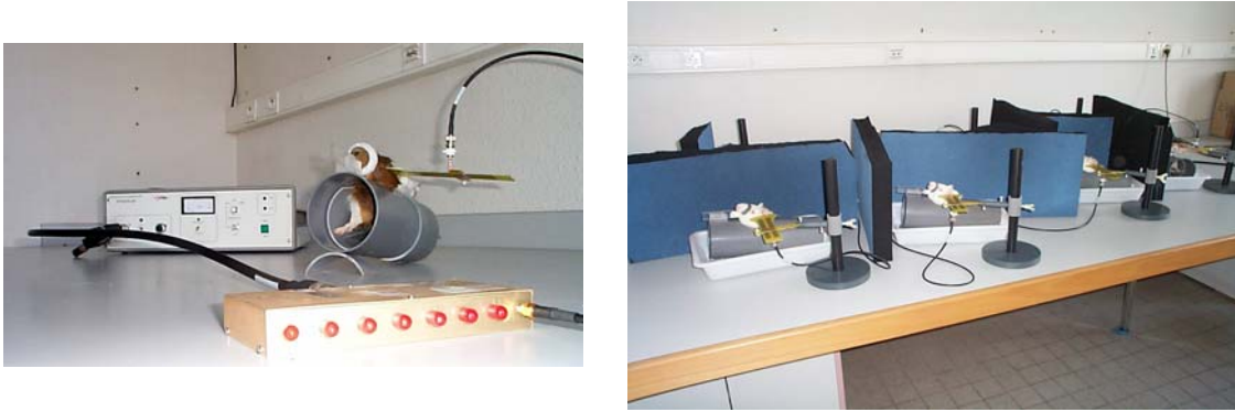
Fig. 2.9 – On the left: Exposure system: the 8-channel divider, the generator and the antenna. On the right: Exposure systems for 8 GPs at a time.
