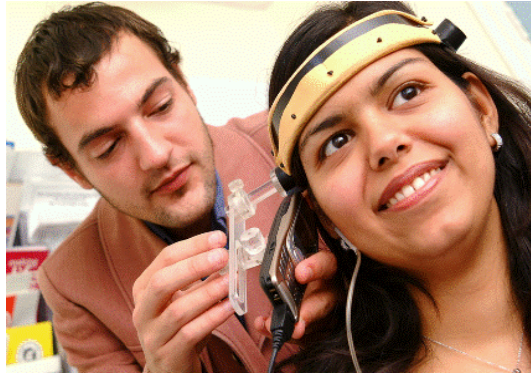
Fig 2.10 Example of exposure system positioning during experiments
