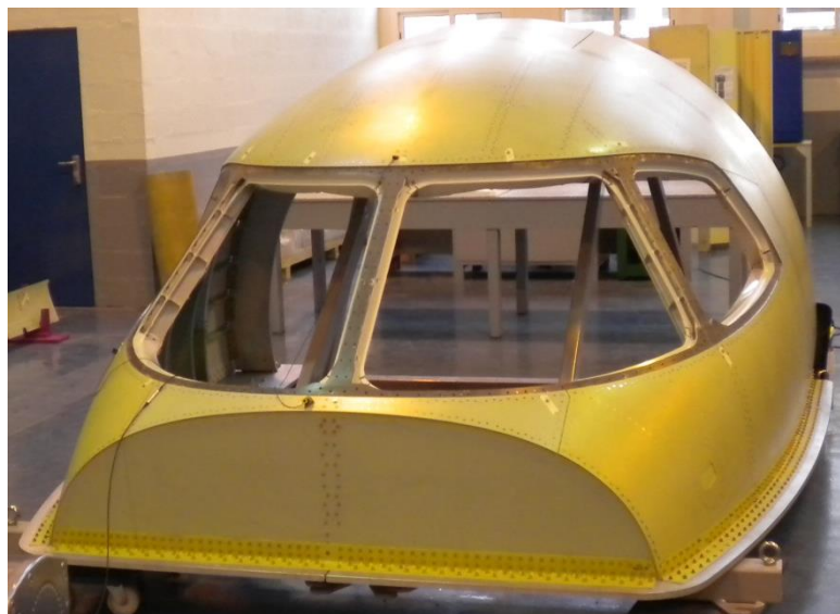
Figure 1: Picture of the 5X Upper T12 coupon (transparencies not installed) used for bird strike and hail tests
