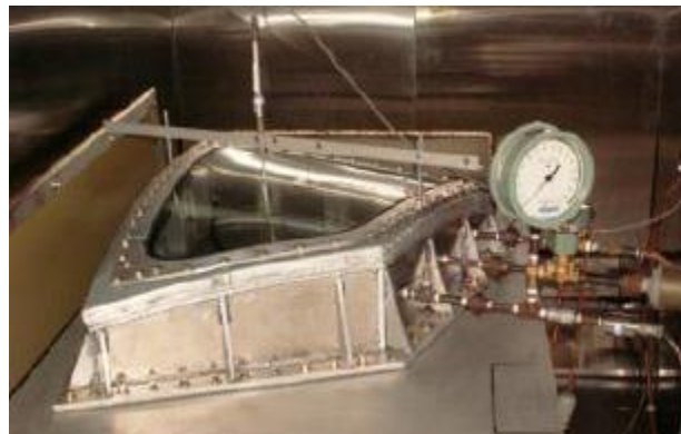
Figure 3: Picture of one of the 5X transparencies during pressure test
