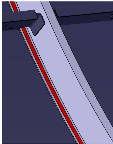
Figure 3: Schematic of a typical Z-profile frame welded against a skin. The rough weld position is shown in red. Note that the position of FSSW would be in regular intervals along this line
