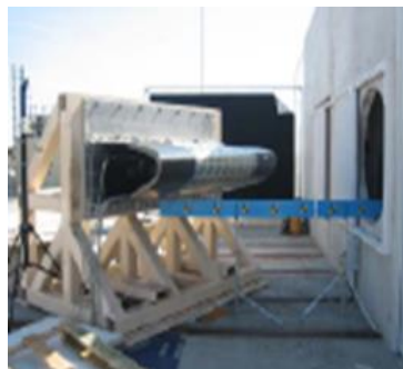
Leading Edge Bird Strike Impact test Simulations and Test Set-Up examples (only as reference)
