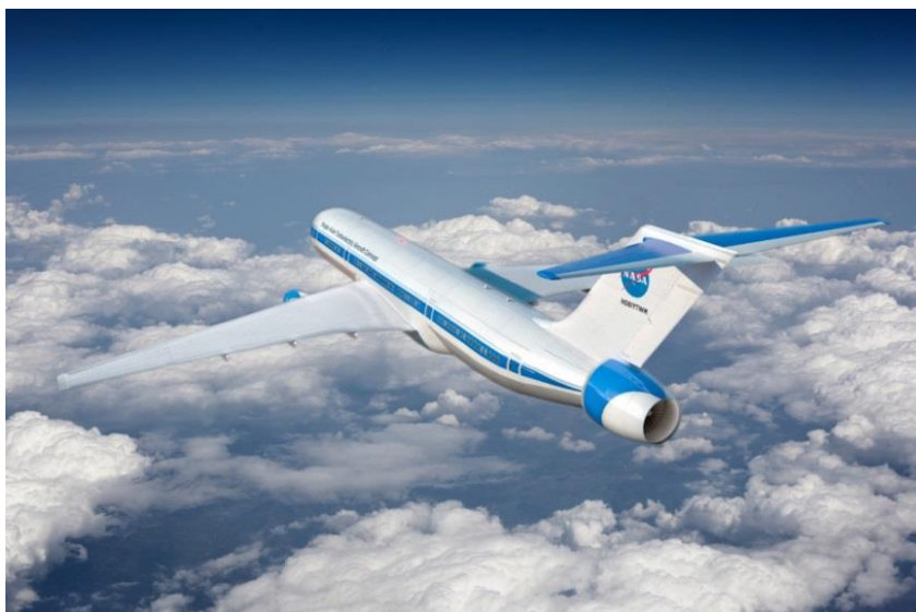
Figure 1 - Propulsive Fuselage – NASA's STARC-ABL turboelectric Plane Concept (NASA, 2018)
