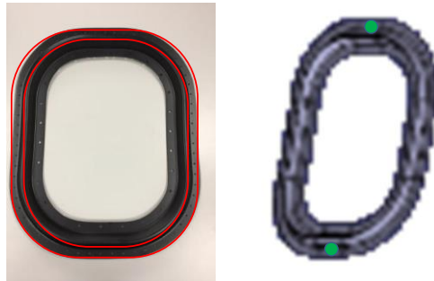
Fig.2. Coordination holes for window frame.
