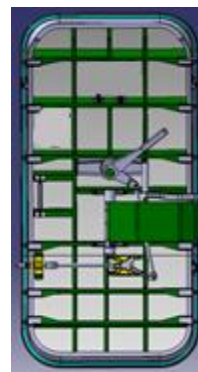
Fig.3 Door Internal structure
