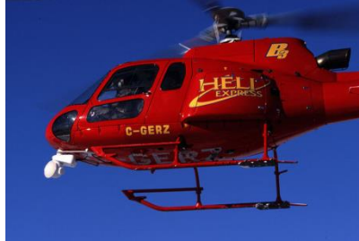
Figure 22: Example of radar based Obstacle Detection Systems installed on rotorcraft
