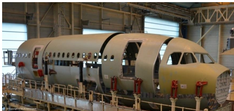
Figure 2: State of the art of half-shell longitudinal joining
