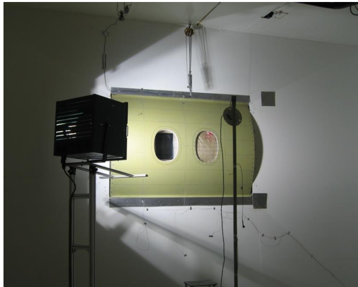
Example of a fuselage panel being tested for light transmission in the acoustic chambers (same installation is used for acoustic tests)
