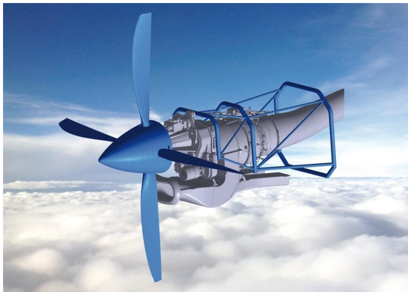
Figure 18: Illustration of Integrated Power Plant System (IPPS)
