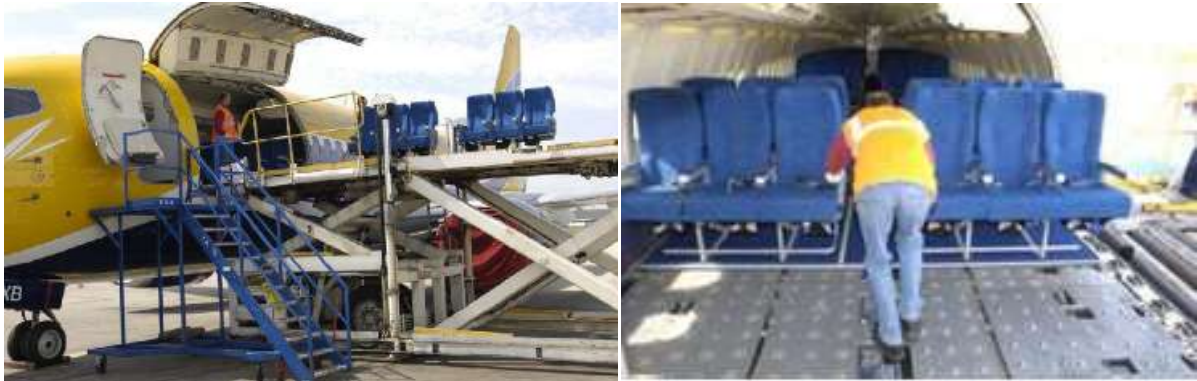
Figure 38: Airplane "Quick change" system
