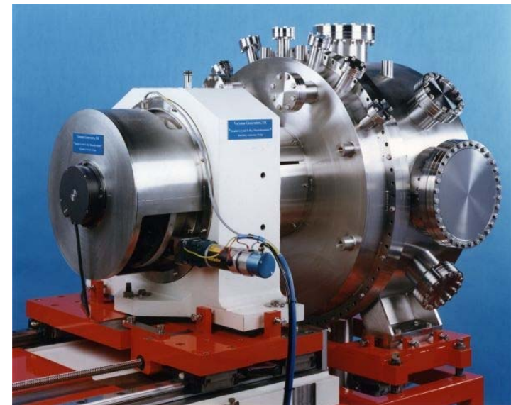
Double-crystal monochromator manufactured by Vacuum Generators in 1995 and delivered to the new Advanced Photon source
