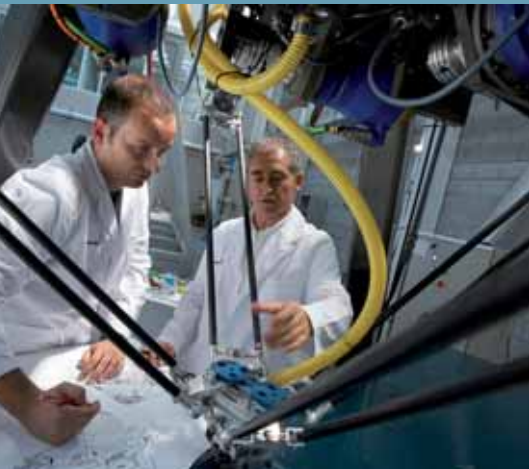
High speed parallel kinematic (PKM) robot for pick-and-place tasks developed in collaboration between FATRONIK-Tecnalia and LIRMM (CNRS).
