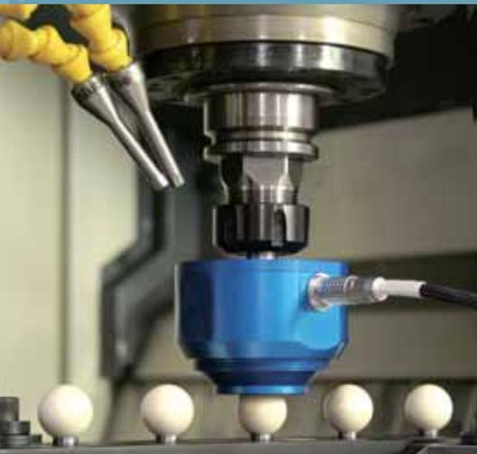
A probe head senses the 3D position of precision balls mounted on a calibrated ball beam, simultaneously measuring machine axis positioning and straightness with  $\mu\text{m}$ -level accuracy.
