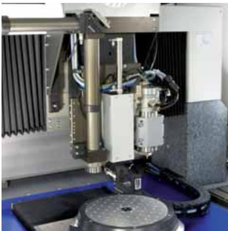
The modular design of the LAUNCH-MICRO machine will permit configuration for three, four or five motion axes, enabling users to keep starting costs low while permitting them to upgrade and adapt their systems to meet developing demands. It can be optimised for pure micromilling, pure ultra-short pulse laser processing, or a combination of the two technologies in one machine platform and CNC-system.
