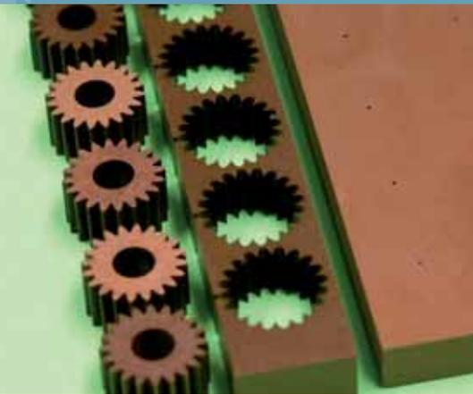
Using W-EDM, complex ceramic components are made flexibly and with great accuracy from a simply shaped ZrO<sub>2</sub>-TiN block. Since no molds are needed, this allows Maxon Motors to decrease lead times and reduce costs for small series production, and to optimise early prototypes before going to mass production.
