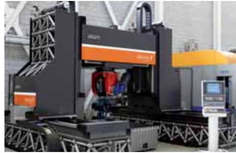
An eco-efficient five-axis machine for friction stir welding (FSW) processes.
