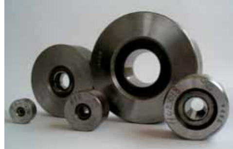
Manufacture of drawing dies in a new range of extremely hard and wear-resistant ceramics gives increased lifetimes.
