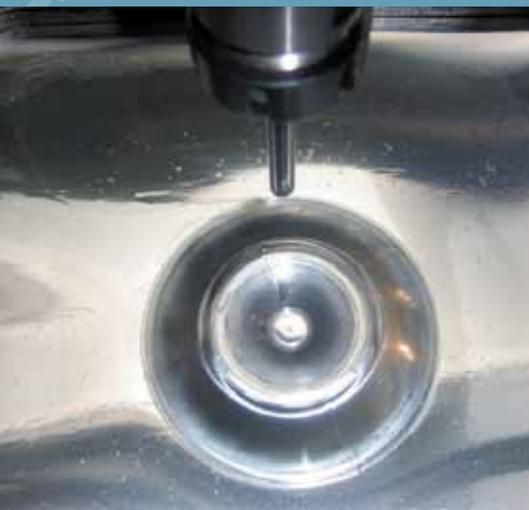
In the SCULPTOR prototype, two opposed tools allow incremental forming of sheet metal parts with no dedicated die. One tool acts as the forming device, while the other provides support. These roles can be interchanged in order to combine convex shapes with concave cavities in the same component.
