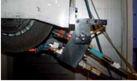
DANOBAT minimum quantity lubricant demonstrator system integrated in a machining centre for grinding.
