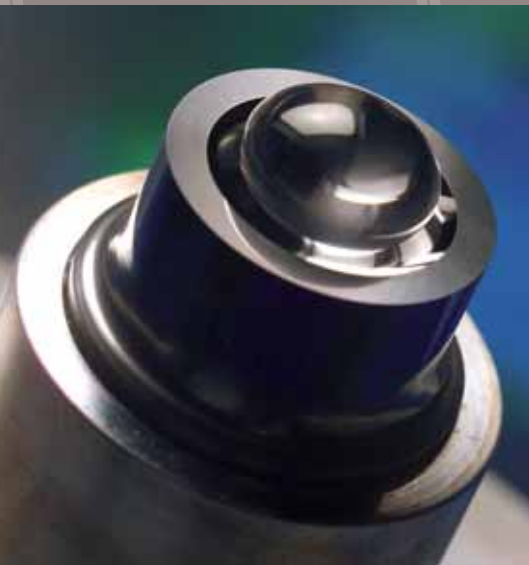
Glass preform in moulding setup ready for the process to start.
