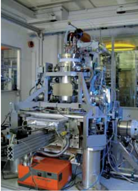
Projection Mask-Less Patterning proof-of-concept tool.
