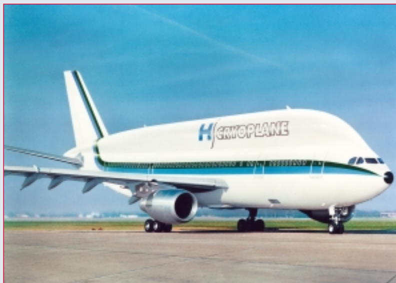
Storing of large volume of liquid hydrogen in insulated containers causes changes in aircraft configuration.
