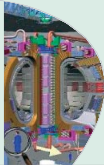
A cut-away drawing of the ITER tokamak
