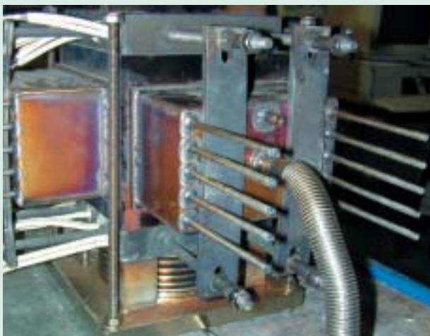
Molten carbonate fuel cell fuelled by biogas (Courtesy of MTU).
