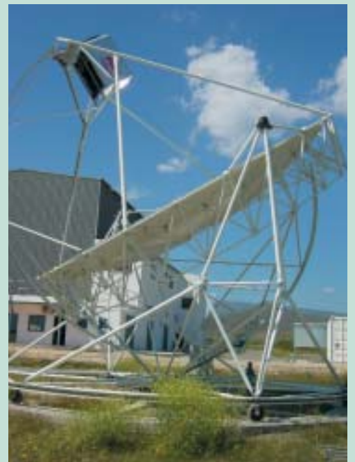
This parabolic dish, from the Eurodish project, with a reflective inner surface can produce up to 10kWe with a Stirling engine located at its focal point (Courtesy of Ph. Schild).
