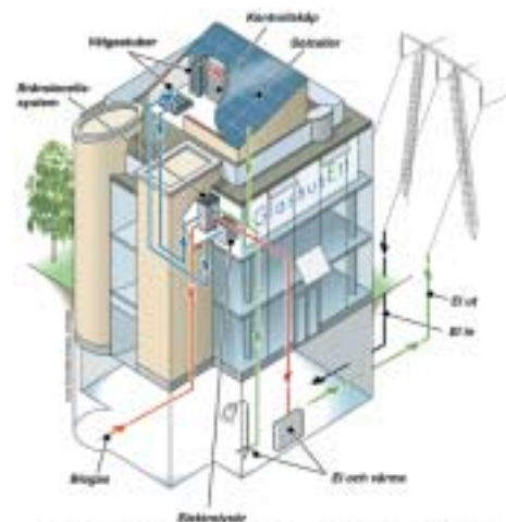
Figure 1: Hydrogen-powered "clever" building operated by ABB in Stockholm.
