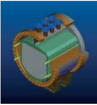
Figure 2: 500 kW, 30 bar PME Test Unit, 0,8m 2 cell area.
