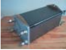
State-of-the-art at the start of the project: an IRD Fuel Cells A/S 500 W DMFC stack.
