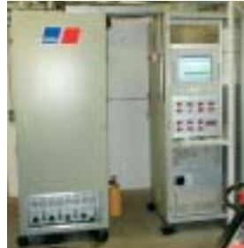
Figure 2: MCFC Testbed (left MCFC unit, right controlling unit) at the Seaborne premises.
