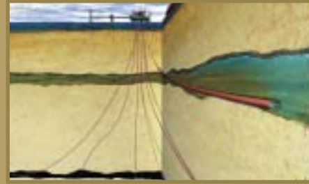
CO 2 injection in deep saline aquifers
