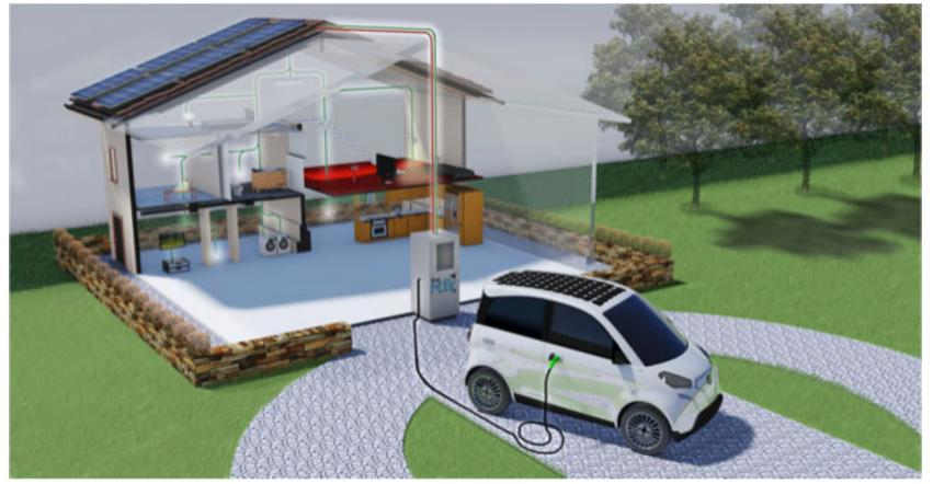
Multidirectional energy exchange between grid-home-stationary rack energy storage - renewable energy installation and electric vehicle. Also including the demonstration of partial battery swapping between EV and stationary energy storage rack (Source: ICT-FREE-MOBY and PLUS-MOBY projects).
