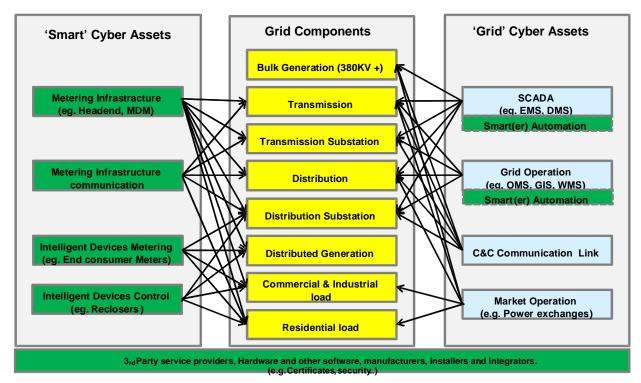
Smart grid is an evolutionary theme. It is built on the existing (core components) and introduce various new functions and capabilities (in green) to the core components.
