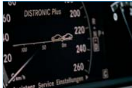
Advanced cruise control systems use radar to help drivers maintain a safe distance
