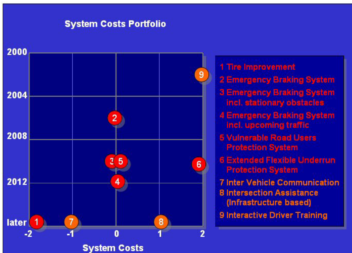
Fig. 8: System costs of effective approaches towards enhanced road safety performance for heavy duty vehicles.
