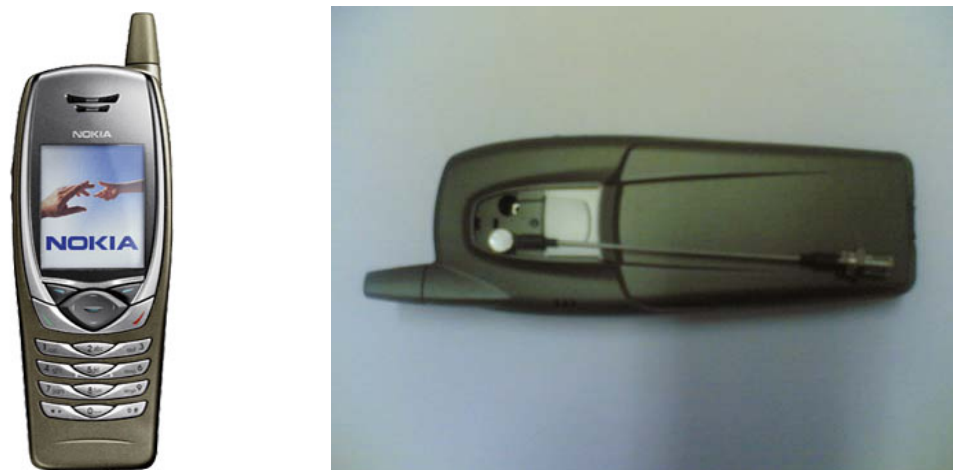
Fig.1. Power measurements and the external RF output and cable on the Nokia 6650 phone
