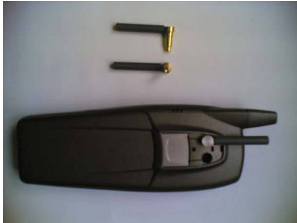
Fig.9 External load and dummy load connected to the external RF output on the backside of Nokia 6650 phone
