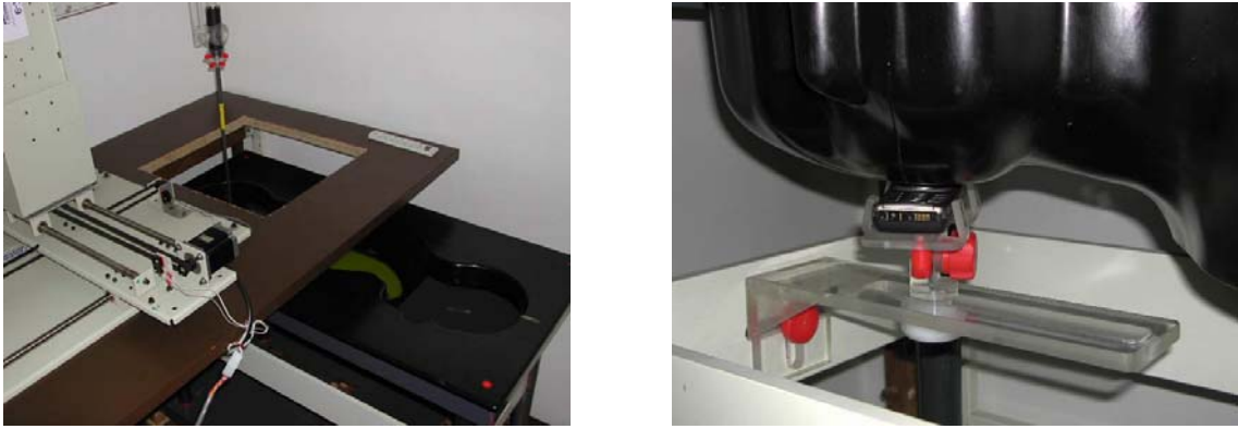
Fig.7. SAR measurement system with liquid phantom and 3D motor driver system.
