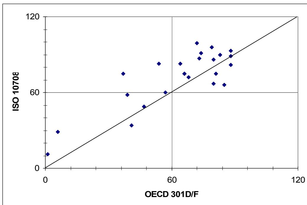
Using the biodegradability pass criterion of the 60% BOD/COD, comparison of the biodegradability test data of 24 surfactants shows that 21 compounds (88%) reached the same evaluation (14 above and 7 below the pass level) whereas 3 compounds (12%) only passed the ISO-10708 test.
