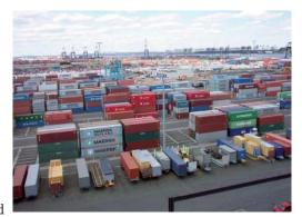
Containers are normally 8 foot height but other heights also exist." High cube containers" are containers with a height of 9.5 foot." Super high cube containers" are containers exceeding the ISO dimensions. They include container lengths of 45 foot, 48 foot and 53 foot.
