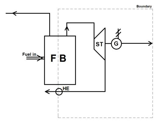
The boiler feeding heat or steam into the CHP unit is also providing heat or steam for an installation outside the CHP unit (e.g. steam for industrial customers). As this heat/steam never enters the turbine of the CHP unit), this heat/steam is called reduction heat ( $H_{reduction}$ ). The relevant fuel ( $F_{reduction}$ ) to create this heat/steam needs to be excluded from the CHP unit.
