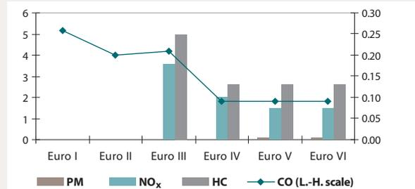
**Figure 7.29:** Diesel LCV > 1.76 t, max 3.5 t, g/km
