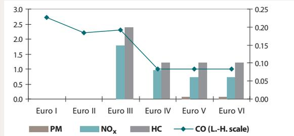
**Figure 7.28:** Diesel 1.76 t > LCV > 1.305 t, g/km
