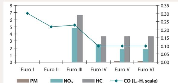
**Figure 7.30:** Diesel, heavy-duty engines, g/kWh
