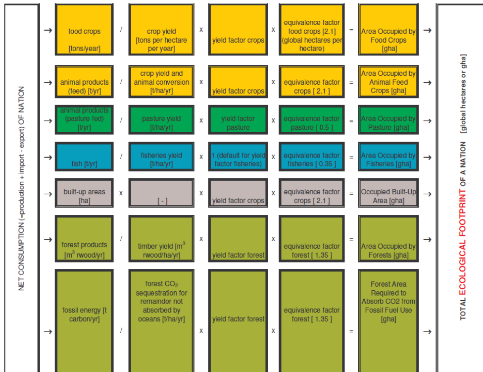
Figure 2-10: Structure of the national Ecological Footprint calculation methodology based on Global Footprint Network 45
