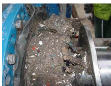
Accumulation of waste in a feed screw
