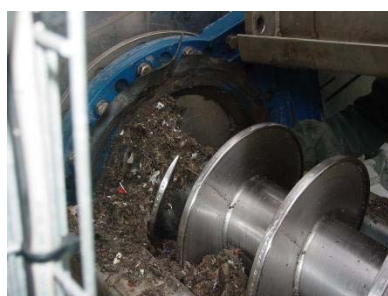
Detail of wear on a feed screw
