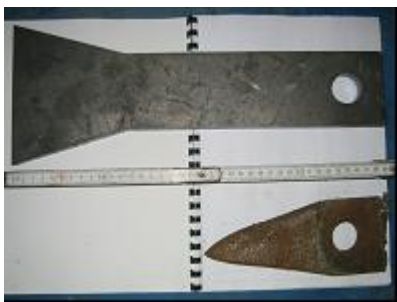
Detail of wear on a mill blade
