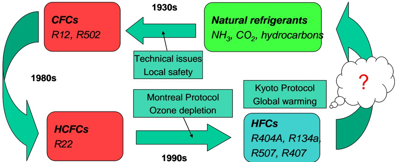
Figure 1: Refrigerant cycle.
