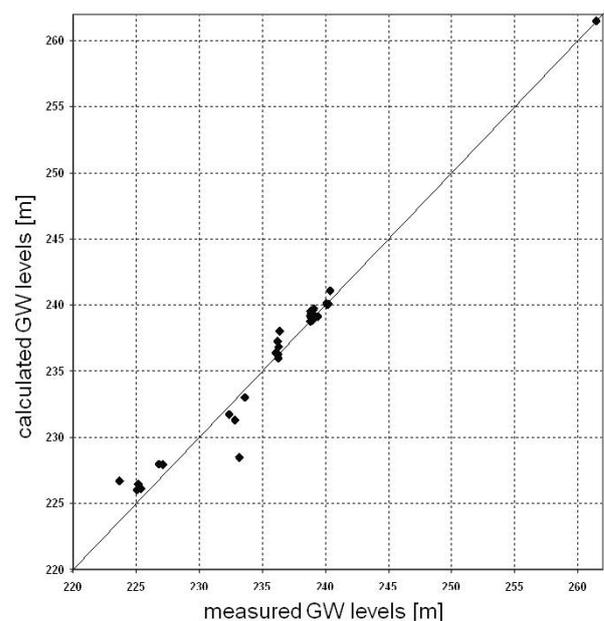
**Fig. 5** Calibration results of piezometer heads (m a.s.l.) in karst aquifer.
