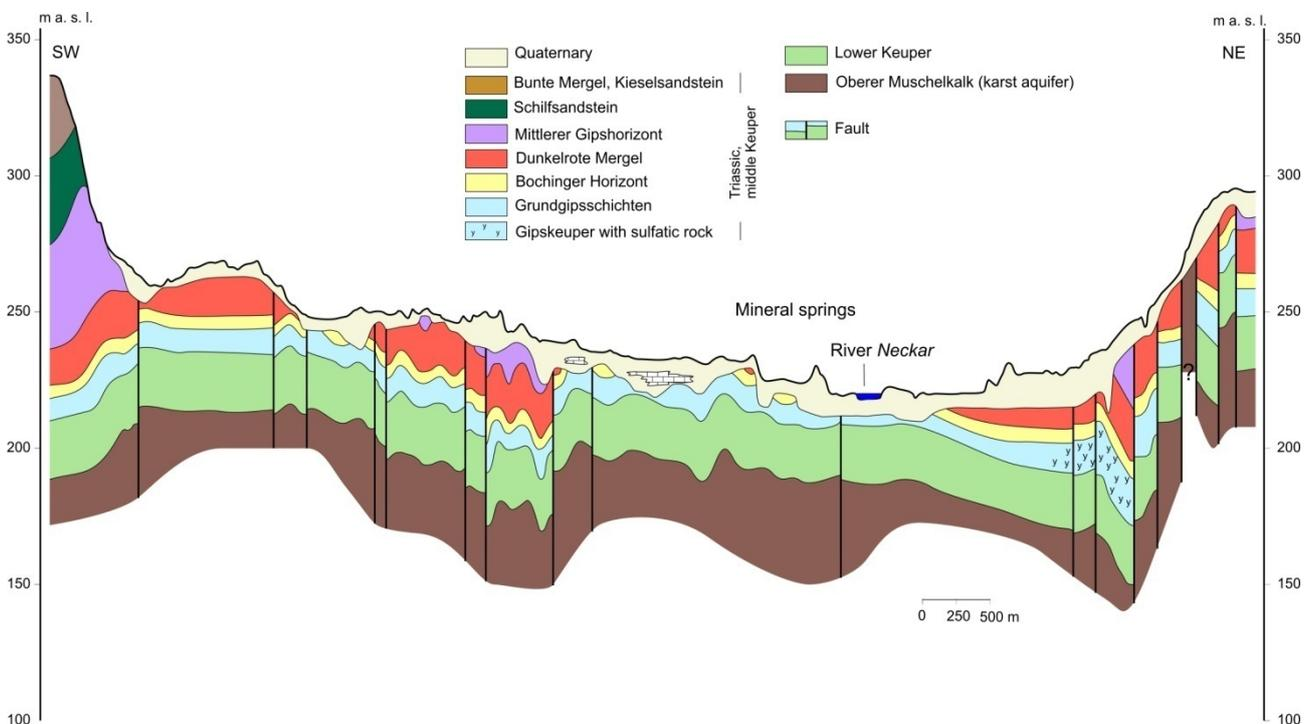
Fig. 2 Geological structuring of aquifers.
