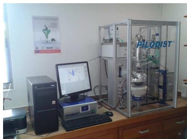
**Picture 2: Vacuum Distillation apparatus**
