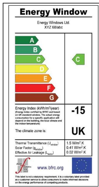
The UK building regulations Part L (for England and Wales) make use of this classification scheme by stating the minimum level for replacement domestic windows is band E while for windows in new domestic extensions, the minimum requirement is band D. In Scotland the matter is discussed in Technical Handbook, Section 6 concerning the energy use of dwellings.<sup>85</sup>
