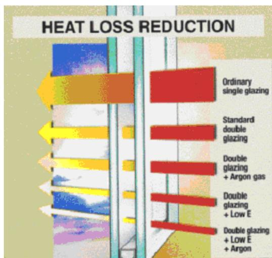
The above diagram illustrates the insulative properties of various types of glazing. For typical U-values for various types of glazing see Table 2 in Section 4.
