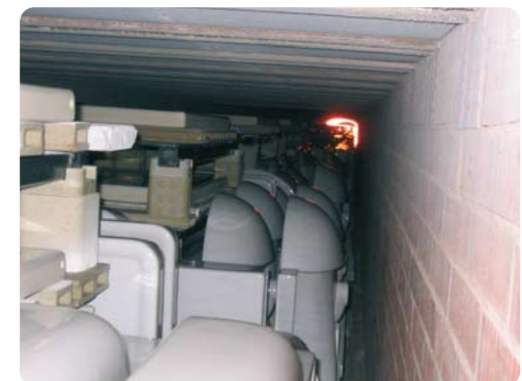
When leaving the post-burning oven, sanitary ceramics have contributed to savings of up to 6.5 % savings in natural gas consumption. Better programming of the heaters helped in setting off the costs which have resulted from the increase of gas prices in 2006.
