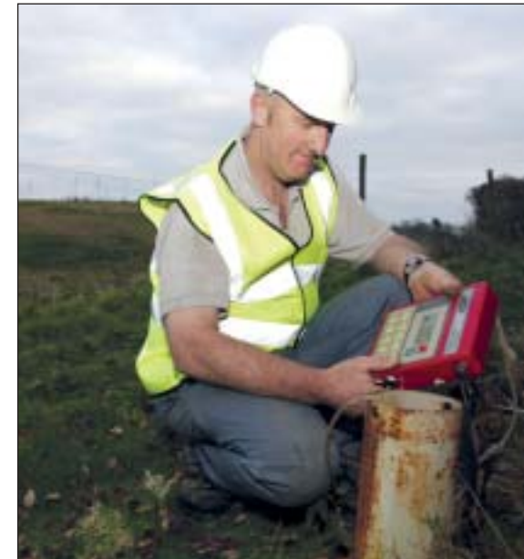
Gas monitoring in bore holes. Patrick Eden
