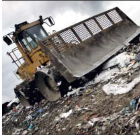
A compactor working on Standen Heath landfill. Patrick Eden
