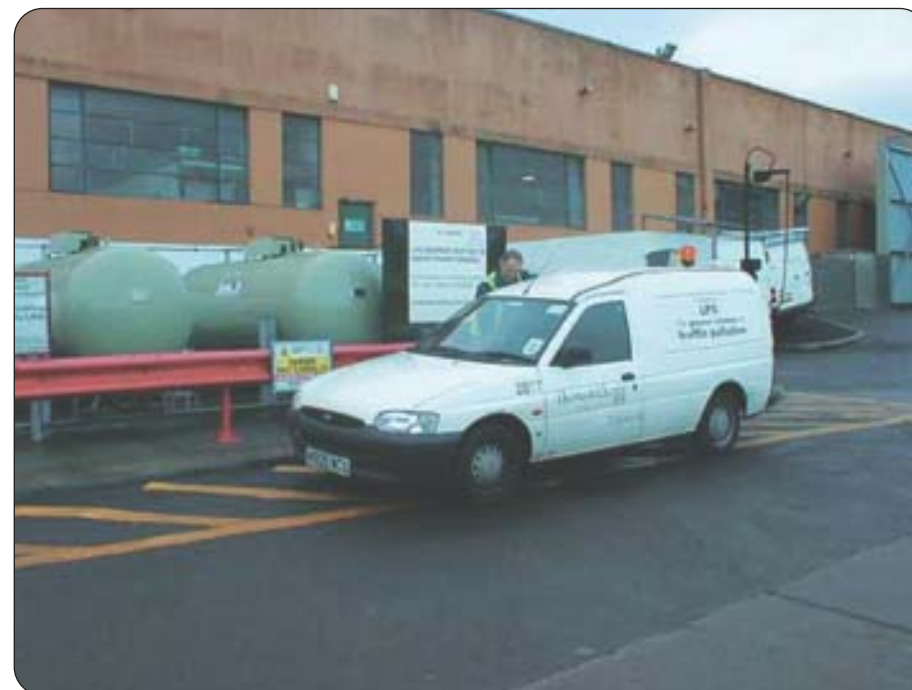
Vehicle filling up with liquid petroleum gas (LPG) from the tanks in the depot.
