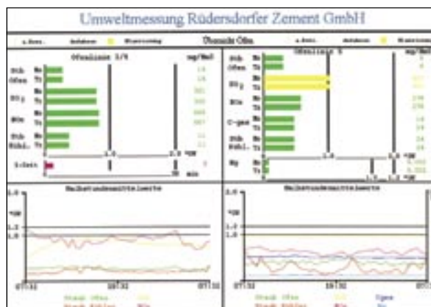
The results of the continuous emissions monitoring are showed on the control panel and are also recorded.
