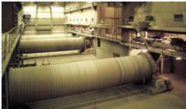
The final grinding of the cement has a positive effect on the working properties.
