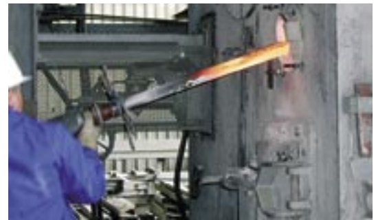
Injection of hydrated lime in the kiln system
