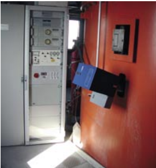
A view of the measuring platform at the stack of kiln line 5, and a look inside showing the emission monitoring system
