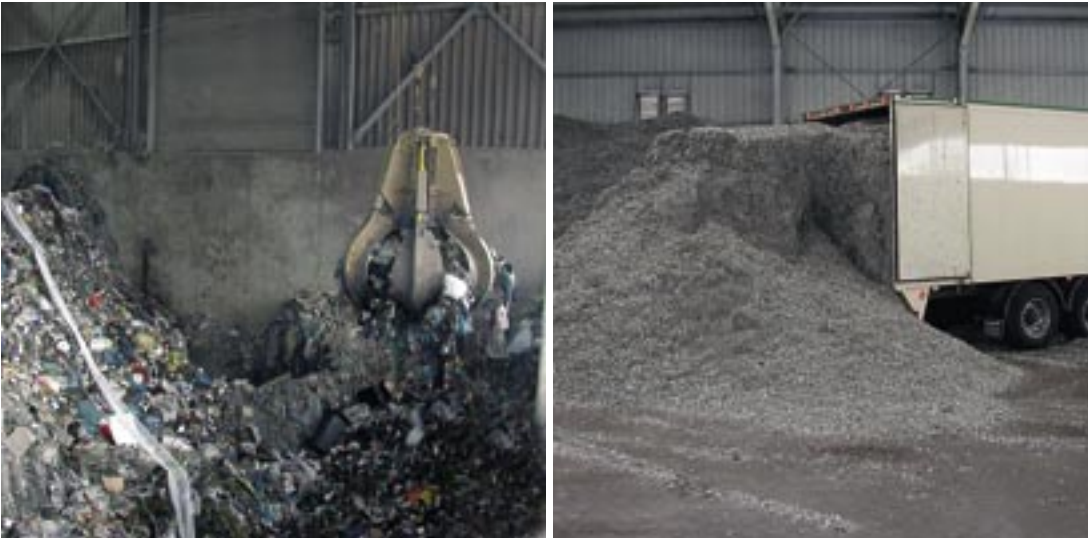
A comparison of the raw waste before preparation (left) and the secondary material as it is delivered to the Rüdersdorf cement works (right).
