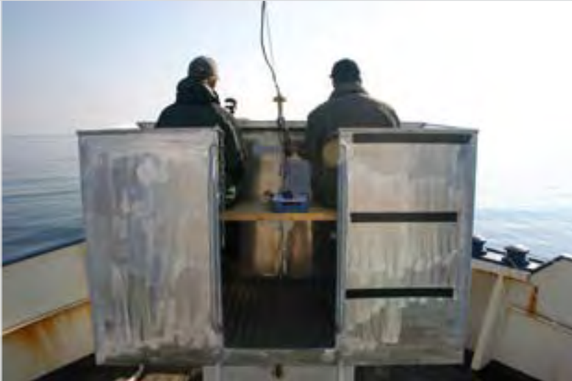
Cetacean observation box installed at the bow of the survey boat
