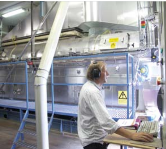
Treating cereal seeds using traditional thermo-techniques.
