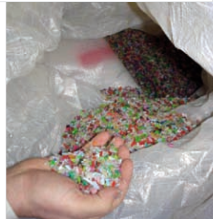
Recycled pellets from thermoplastic waste (e.g. packaging).
