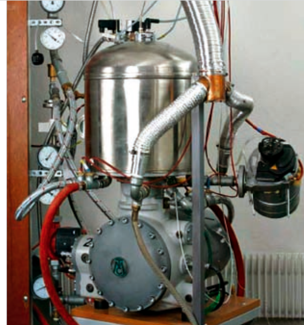
The heart of the cogeneration plant: the 3 kW Stirling engine on its test bench.
