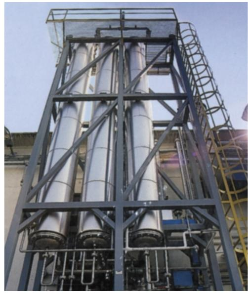
VOCs are first delivered into the outer shell of the condenser, which is wound with a specially designed configuration of spiraled tubes. Liquid nitrogen is released into the emissions vaporising the nitrogen and condensing the VOCs. The gaseous nitrogen is then reused to displace the solvent vapour in the mixers and vessels. Finally the condensed VOCs are collected into an Intermediate Bulk Container (IBC) and reused as solvent for Polychloroprene adhesives.
