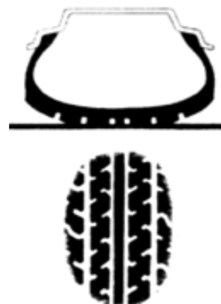
Fig. 2.13: Cross-section and footprint of an over-inflated tyre [12]
