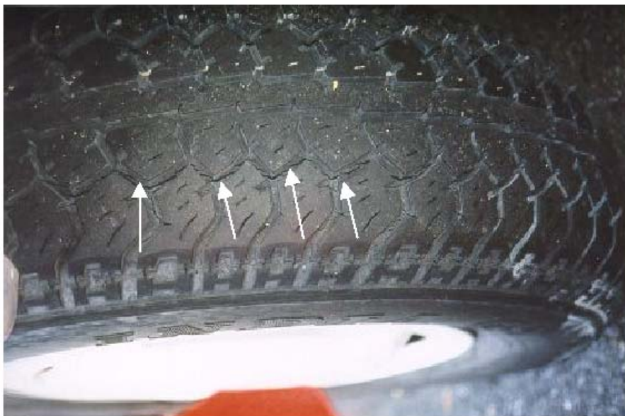
Fig. 2.6: Aging defects (e.g. cracks)
