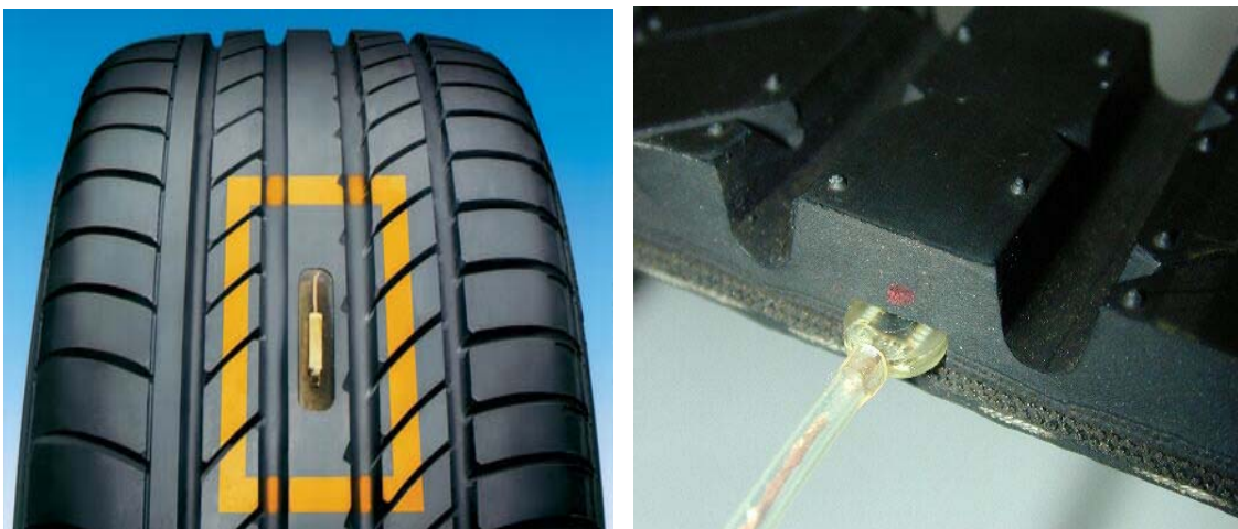
Fig. 3.9 and 3.10: SAW, vulcanised into the tyre tread [24]
