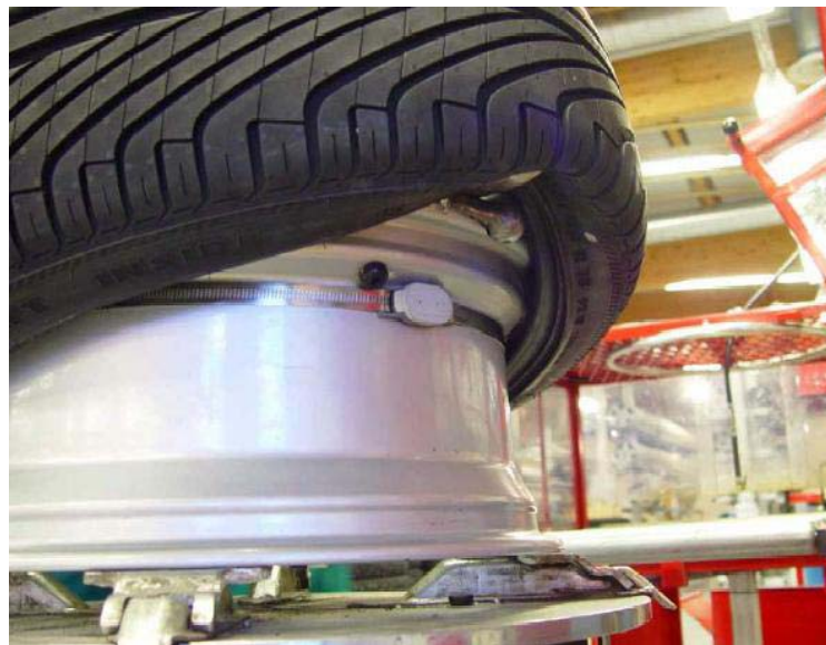
Fig. 3.6: Example of a sensor unit mounted by a steel strap [20]
