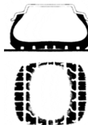
Fig. 2.14: Cross-section and footprint of an under-inflated tyre [12]
