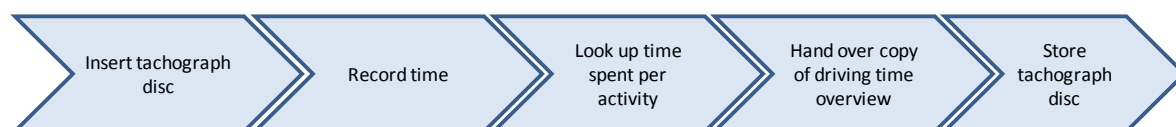
Figure 4: Business process for "Recording time spent driving a vehicle and recording working time, analogue tachograph"
