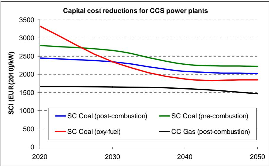
Figure 7.3: Trends in capital costs of supercritical (SC) coal and combined cycle (CC) natural gas power plants with CCS technology (Source: JRC estimates)
